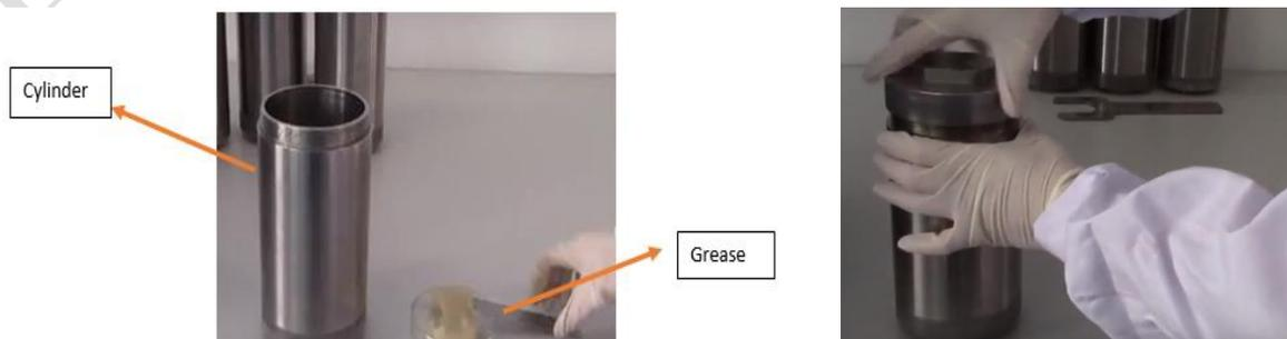
**Figure 5: Grease with cylinder which have to be applied inside**
